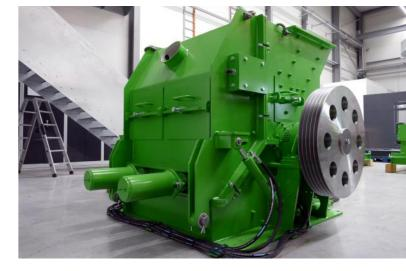
Double feeding enables parallel processing of different input fractions
