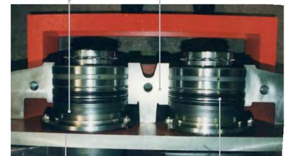
additional bulkhead bearing sealing
